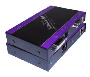
The DVX-PRO extends any DVI-D signal, full duplex RS232 and stereo sound up to 250ft with Cat6 STP cable
