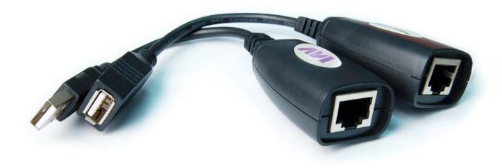
USB-Xpress extends Universal Serial Bus (USB) via a single Cat5 cable. Using a unique method of transparent data transfer, the system allows a USB peripheral to be located up to 150ft from the CPU. Fully compliant with the USB specification, the extender provides a transparent path for both 1.5 and 12 Mbps data.
