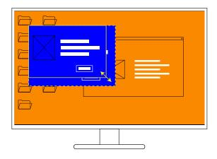
**PIP MODE** : The SAVILayout Mode is a revolutionary feature designed for custom control in your multiviewer KVM. In this mode, the preview mouse, activated by a double-click of the mouse wheel, takes center stage. The preview mouse is your window into channel selection and, in PiP mode, allows for movement and resizing of the smaller thumbnail channel.
