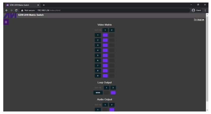
The Matrix Switch page can be used to quickly change individual inputs and outputs for video, loop, and audio. Note: Loop Output 1 and Loop Output 2 only affect the Loop 2/MAIN output. Loop 1 will always display Input 1.
