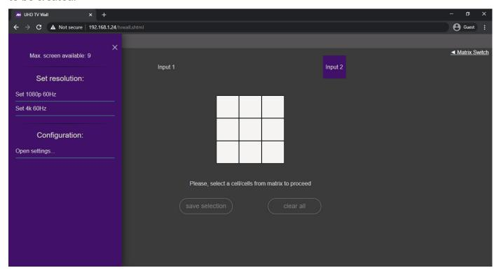
Opening settings allows for the resolution to be changed or open configuration settings.
